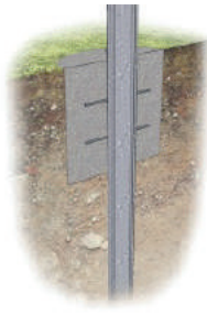
Ramming with concreting
