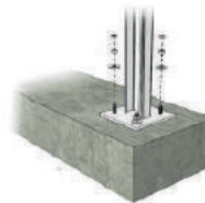
Installation on concrete blocks
