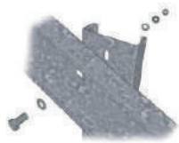
Fastening of main beams to piles
