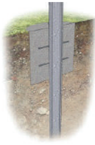
Ramming with concreting
