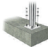
Installation on concrete blocks
