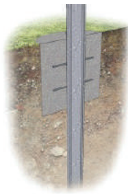
Ramming with concreting
