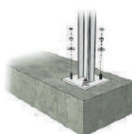
Installation on concrete blocks
