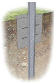
Ramming with concreting
