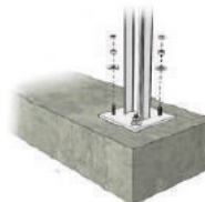
Installation on concrete blocks
