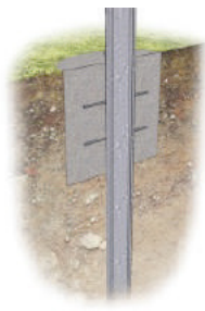
Ramming with concreting
