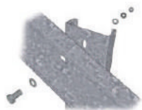
Fastening of main beams to piles
