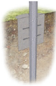
Ramming with concreting
