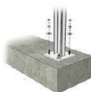
Installation on concrete blocks
