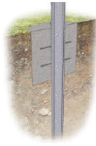
Ramming with concreting
