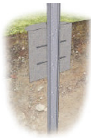
Ramming with concreting
