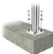
Installation on concrete blocks
