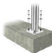
Installation on concrete blocks
